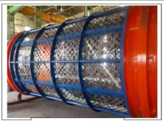
The rejects from the 100mm sieve will be taken to RDF storage area for further processing / sorting. The sorted waste containing mostly the organic portion of the fresh garbage will be taken to the compost pad for windrow formation by reversible conveyors.
